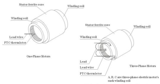
\* Embed thermistor in the coil, see the picture above. Soak it together with the coil, then dry them completely.
